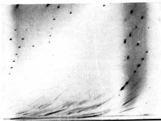
Fig. 4. First layer a -axis Weissenberg photograph of the other face of the crystal taken with \text{Cu } K\alpha radiation on a camera of diameter 5.73 cm.
